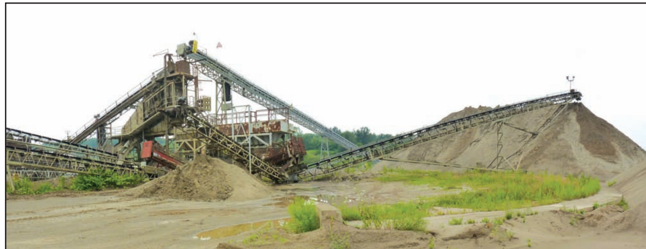
Sand is stacked in a stockpile with a 150-foot Supreme Radial Stacker after it comes from a McLanahan twin screw sand washer. The new overland conveyor is in the center of the photo, terminating atop the processing plant.
