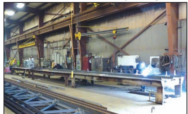
Welders work on support steel as they fabricate new conveyor structures in the Supreme Manufacturing, Inc. plant near Stoneboro, PA.
